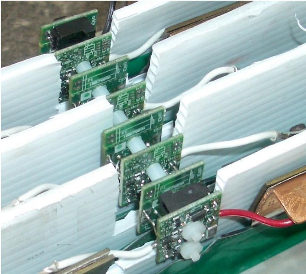
Figure 4.2: Detailed view of cell boards between tabs
