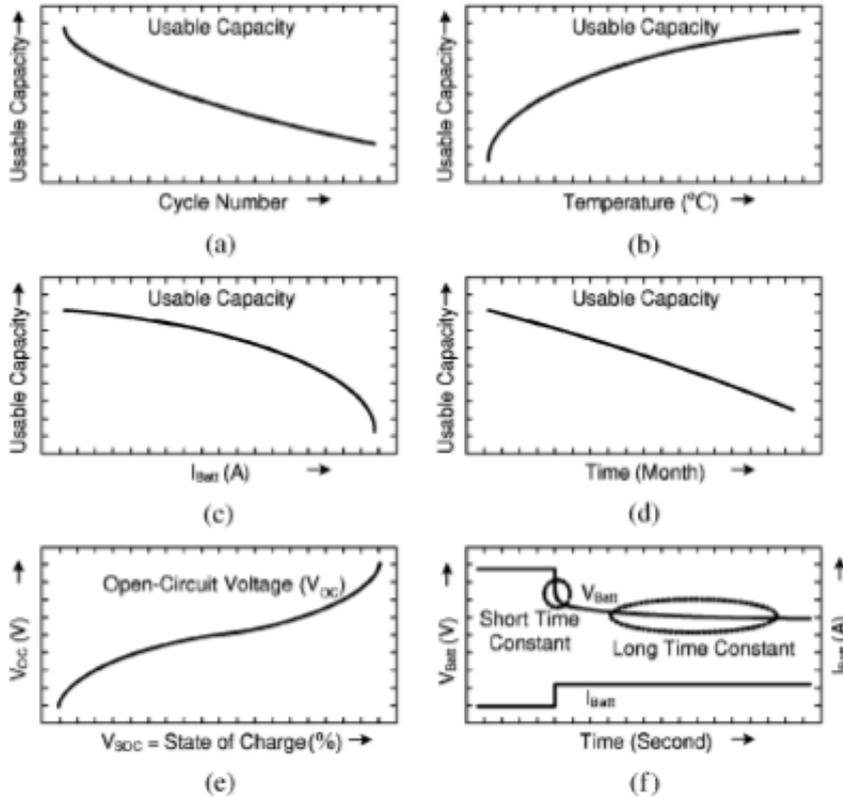
Figure 2.6: Typical battery characteristic curves of usable capacity versus (a) cycle number, (b) temperature, (c) current, and (d) storage time, as well as (e) open- circuit voltage versus SoC and (f) transient response to a step load-current event.
