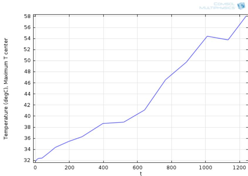
Figure 6.7: Time dependant tempaure of the central cell during the race
