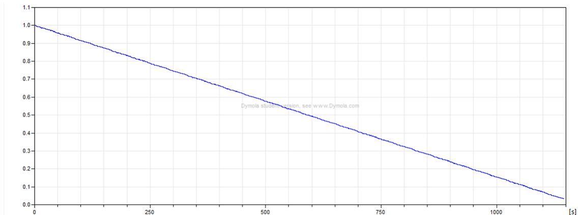
Figure 5.5: SoC simulation with a maximum power limit of 45kW available at the wheels
