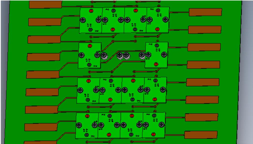
Figure 4.8: Bottom view without 2 cells showing how cells are connected to tracks
