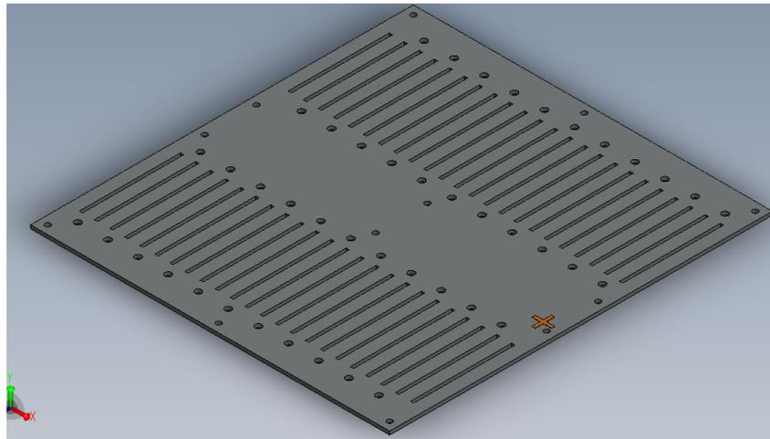
Figure 4.3: Separation layer between cells and electronic circuitry
