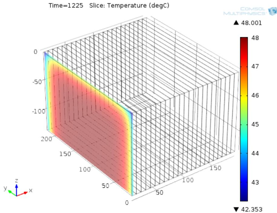
Figure 6.9: Spatial gradient of the leftmost cell at the end of the race
