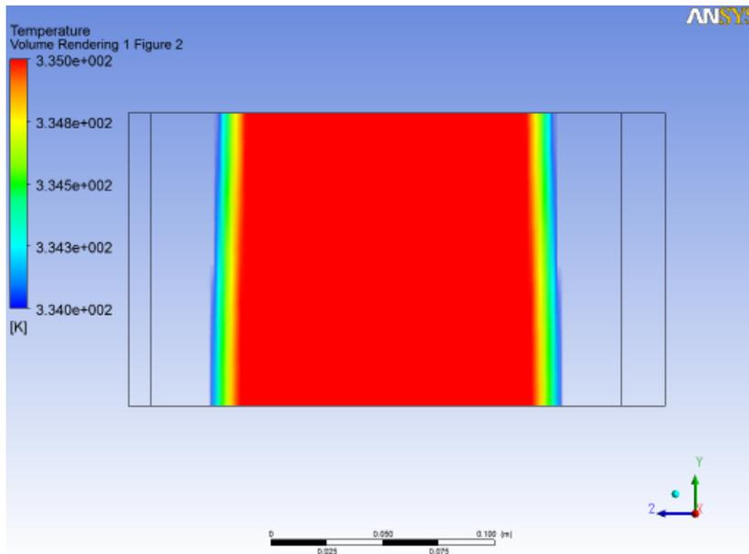
Figure 6.13: Area inside the cell with temperatures between 334 K and 335 K
