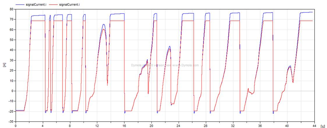
Figure 5.12: Single lap comparison between simplified and run-time calculated currents, at SoC=0,3
