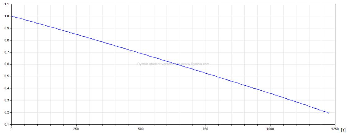
Figure 5.9: SoC simulation supposing a maximum mechanic power limit of 35kW, without constant voltage hypothesis
