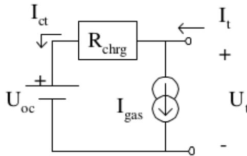
Figure 2.8: Electrical equivalent circuit model of a cell with charging resistance, storage element and gassing current.
