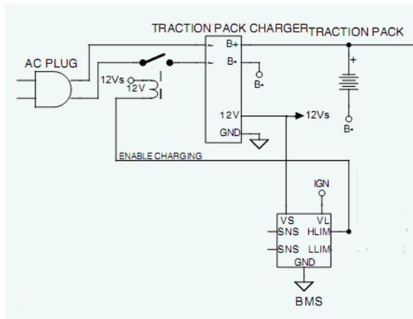
Figure 3.10: Charger-BMS connection during charging phase
