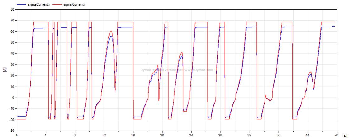
Figure 5.11: Single lap comparison between simplified and run-time calculated currents, with fully charged battery
