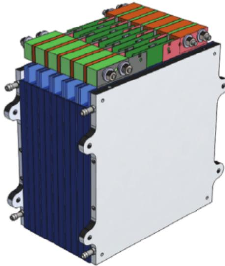
Figure 4.1: Traditional arrangement of pouch cells
