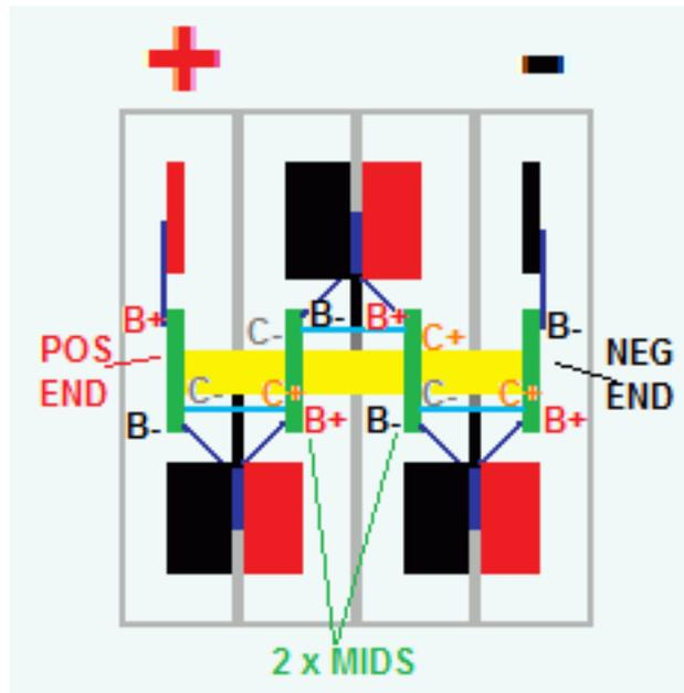
Figure 3.20: Top view of cell stacks, after cells tabs are folded to form series connection.
