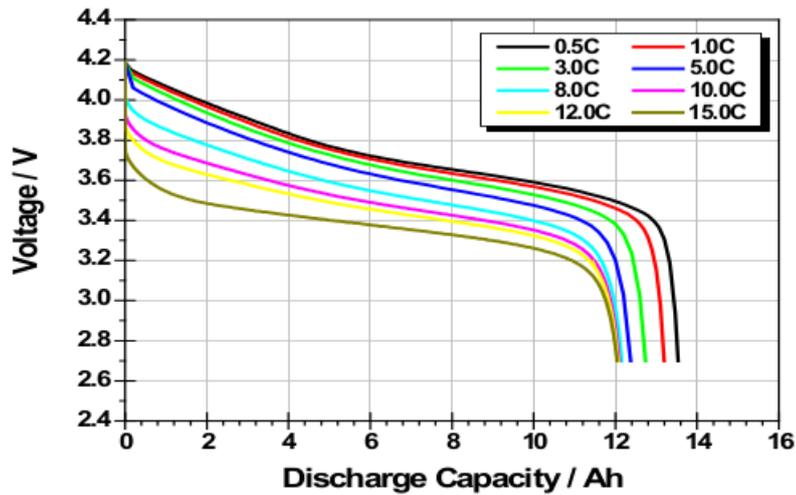
Figure 2.2: Voltage vs. capacity at vary C rates and constant temperature
