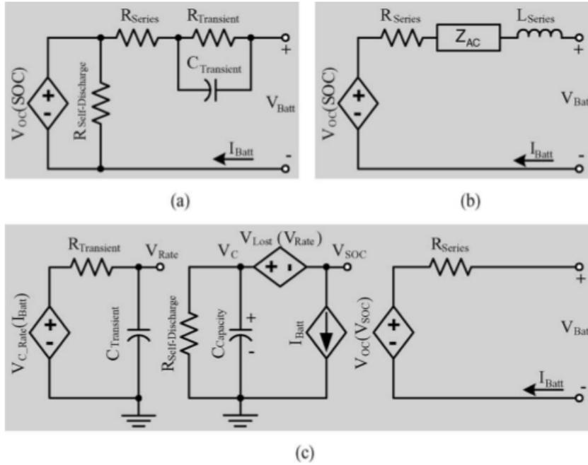
Figure 2.4: (a) Thevenin, (b) impedance and (c) runtime based electrical models
