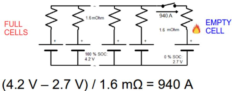
Figure 3.3: Inrush in current due to different voltage levels
