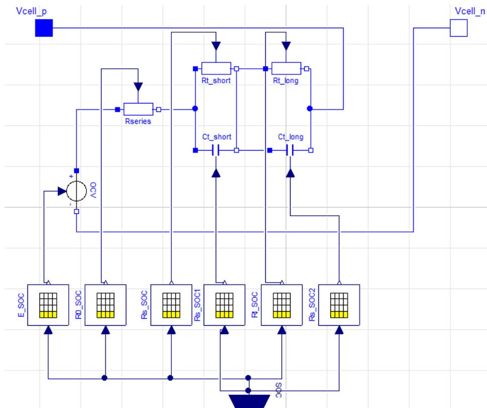
Figure 5.3: Dymola model of a single cell
