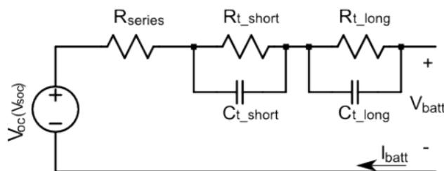
Figure 5.1: Cell electric model
