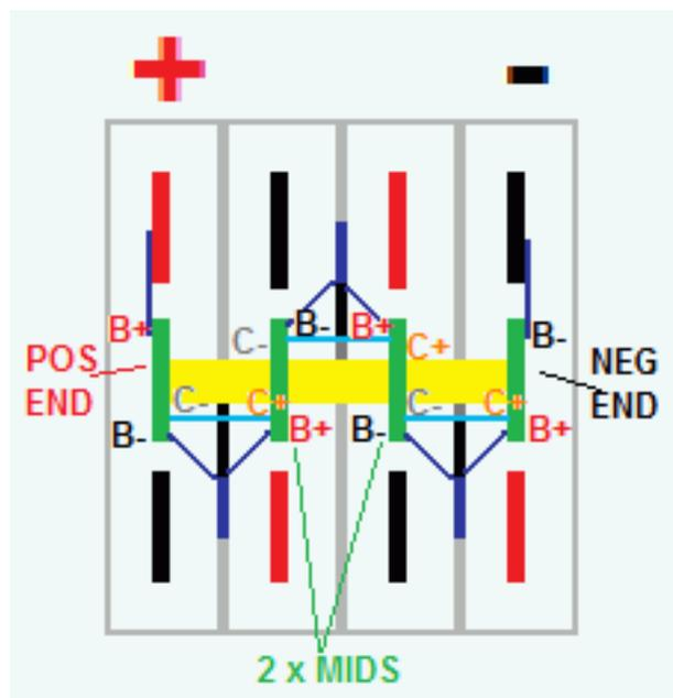
Figure 3.19: Top view of cell stacks, before cells tabs are folded to form series connection.
