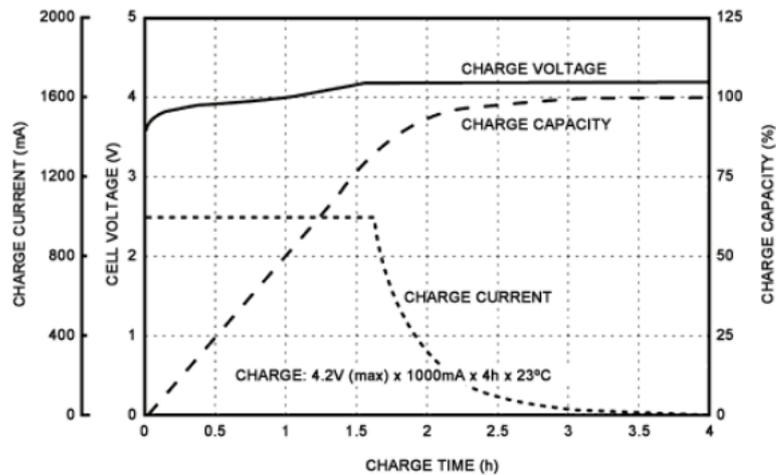
Figure 2.9: Time evolution of CC-CV charge of a Li-on cell.
