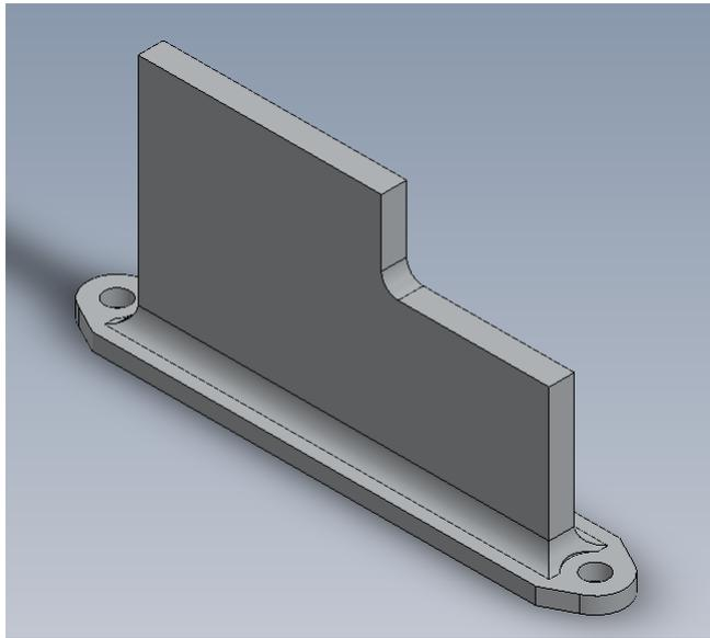
Figure 4.4: Metal bar used as electric connector.
