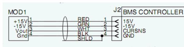
Figure 3.21: Current sensor connections to the BMS controller.
