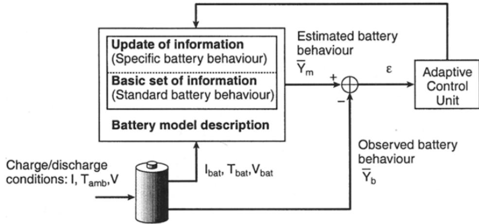
Figure 2.7: Basic principle of an adaptive SoC indication system
