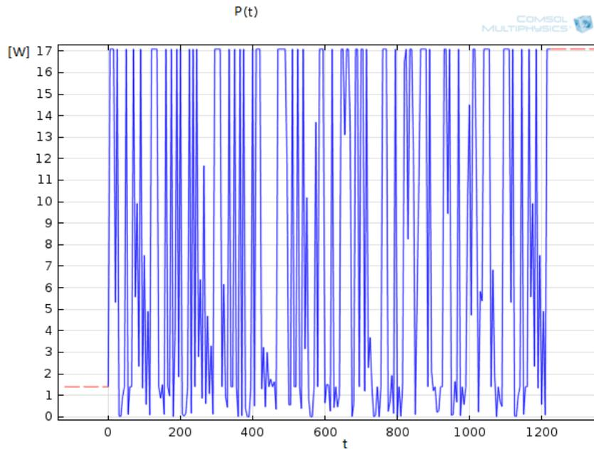
Figure 6.4: Time dependant power wasted as heat by each cell
