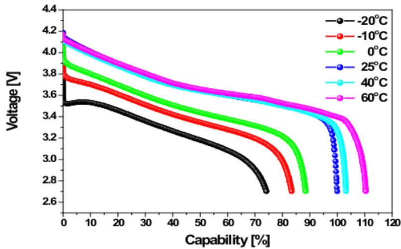
Figure 2.1: Voltage vs. nominal capacity at vary temperature and constant current
