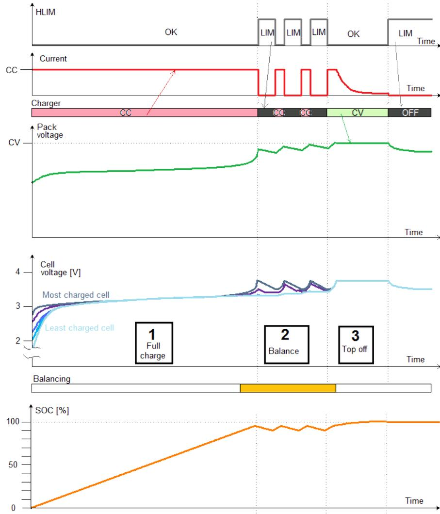
Figure 3.9: Charging phases with constant CC-CV charger and BMS
