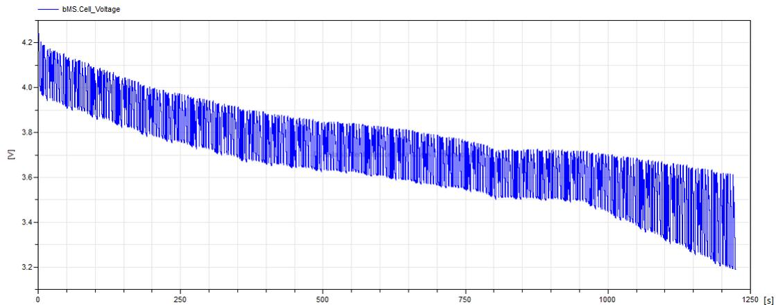
Figure 5.8: Cell voltage variations during a race supposing a maximum power limit of 35 kW available at the wheels
