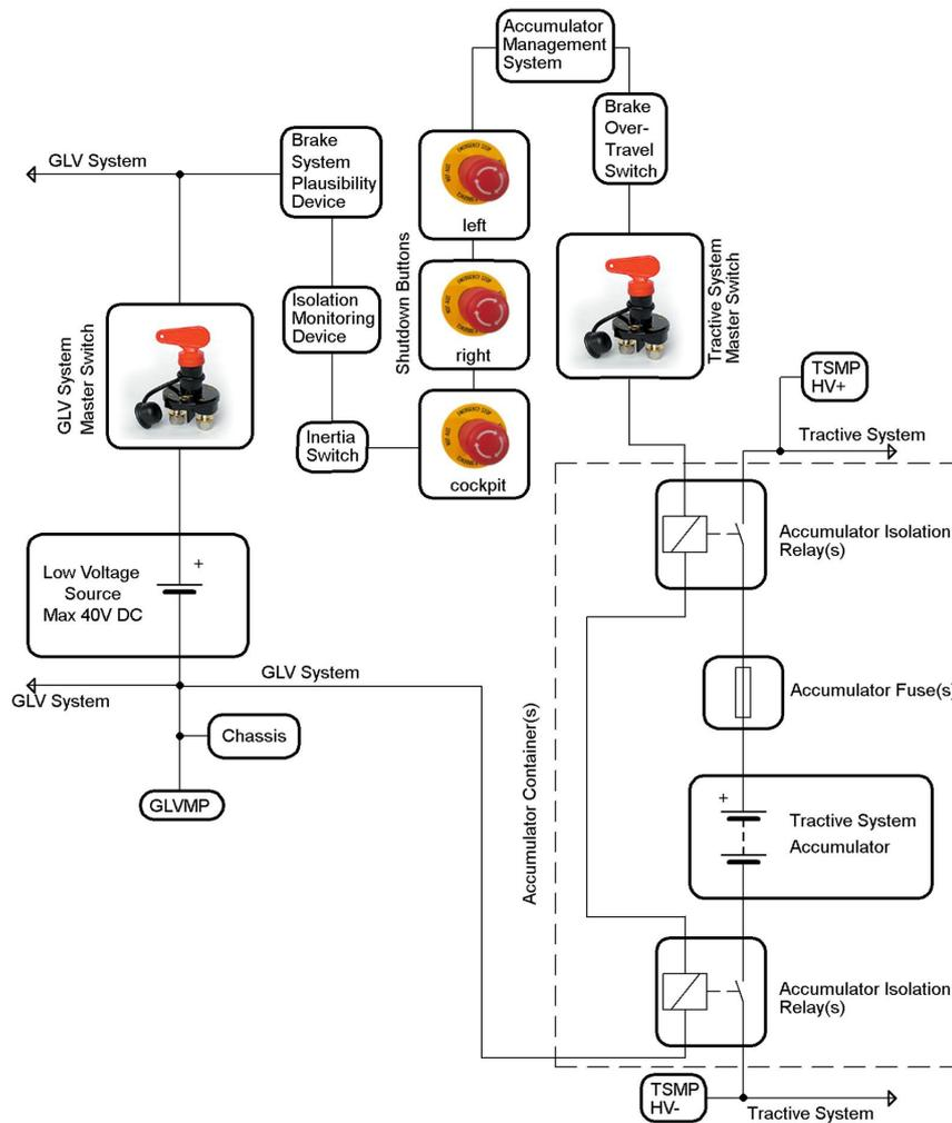
Figure 2.11: Shutdown circuit diagram
