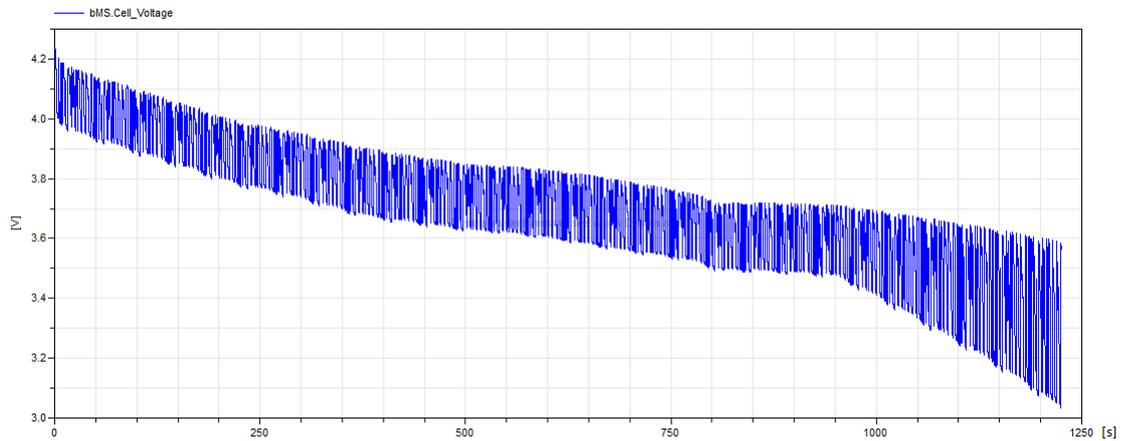
Figure 5.10: Cell voltage variations during a race supposing a maximum mechanic power limit of 35kW, without constant voltage hypothesis
