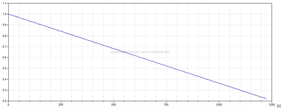
Figure 5.7: SoC simulation with a maximum power limit of 35kW available at the wheels
