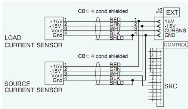
Figure 3.22: Two current sensors connections to the BMS controller.
