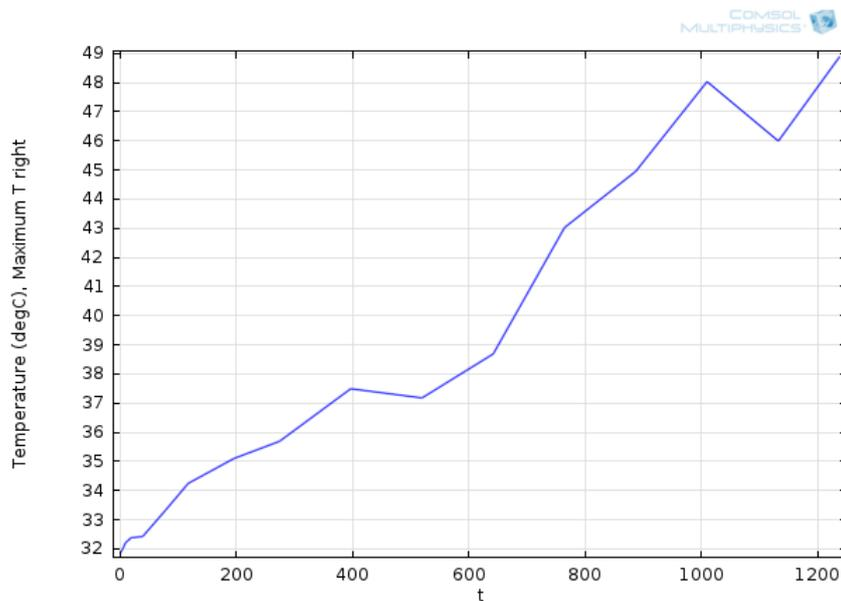
Figure 6.8: Time dependant temperature of the rightmost cell during the race
