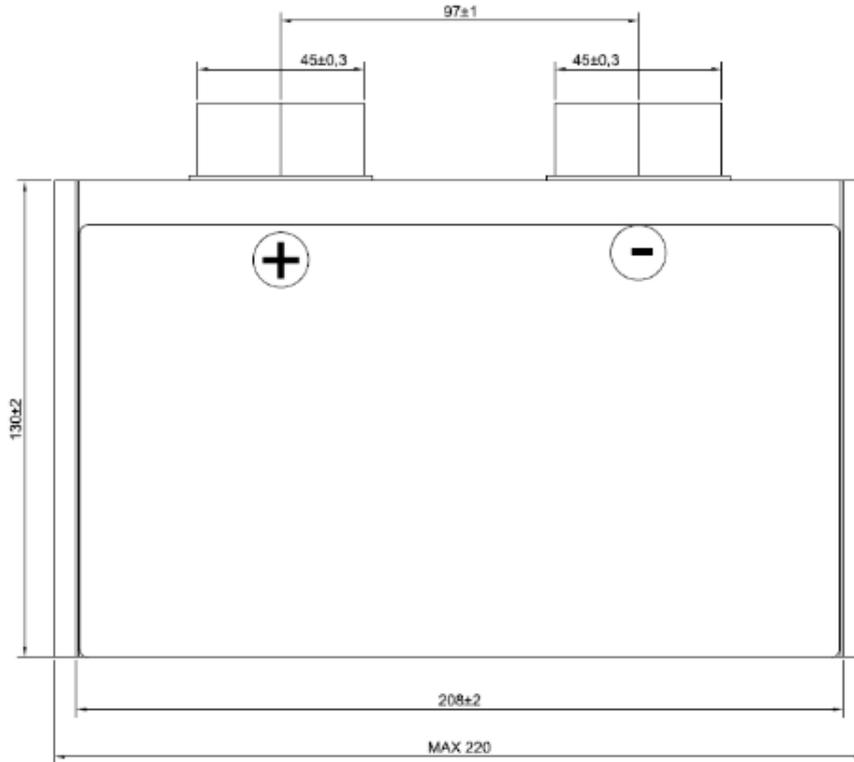
Figure 6.5: Kokam SLPB70205130P two dimensional drawing
