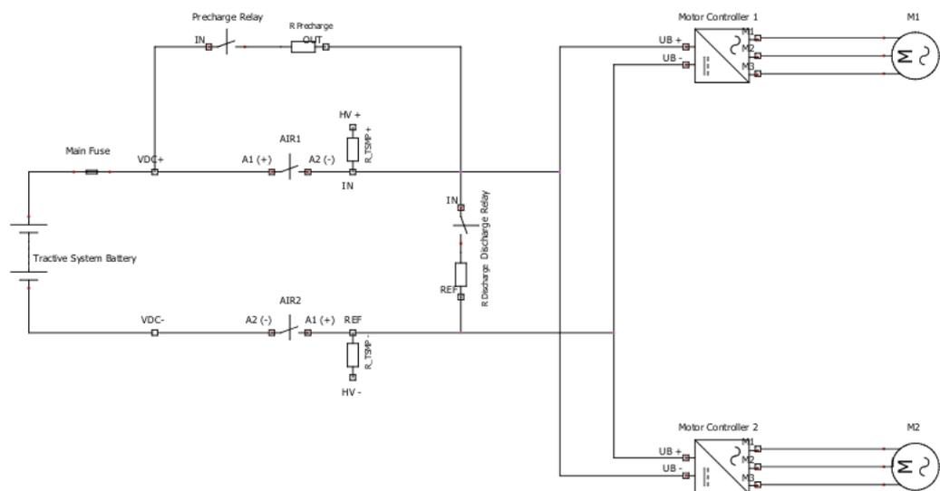
Figure 3.23: Electric schematic of the whole traction system
