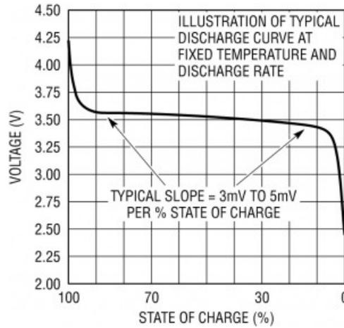
Figure 2.3: Voltage vs. SoC at constant C rates and temperature
