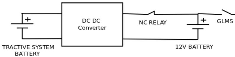
Figure 3.11: Main battery and DC DC converter connection
