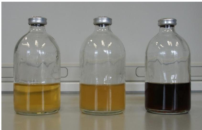
**Fig. 3.1** – Batch cultures in anaerobic state ready to use. From the left, modATCC 1977 added respectively with glucose, milk whey and sugar beet molasses.
